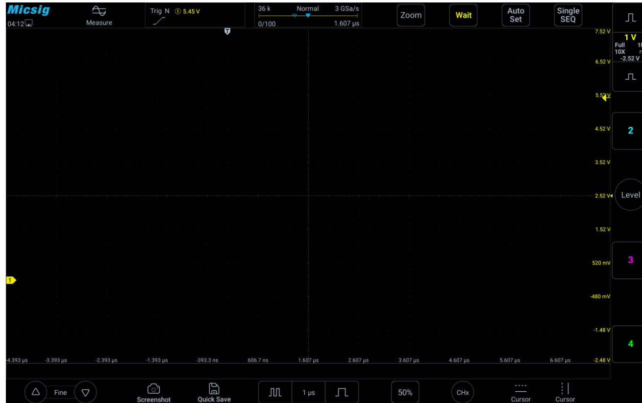
Figure 10-14 Single trigger segmented storage
