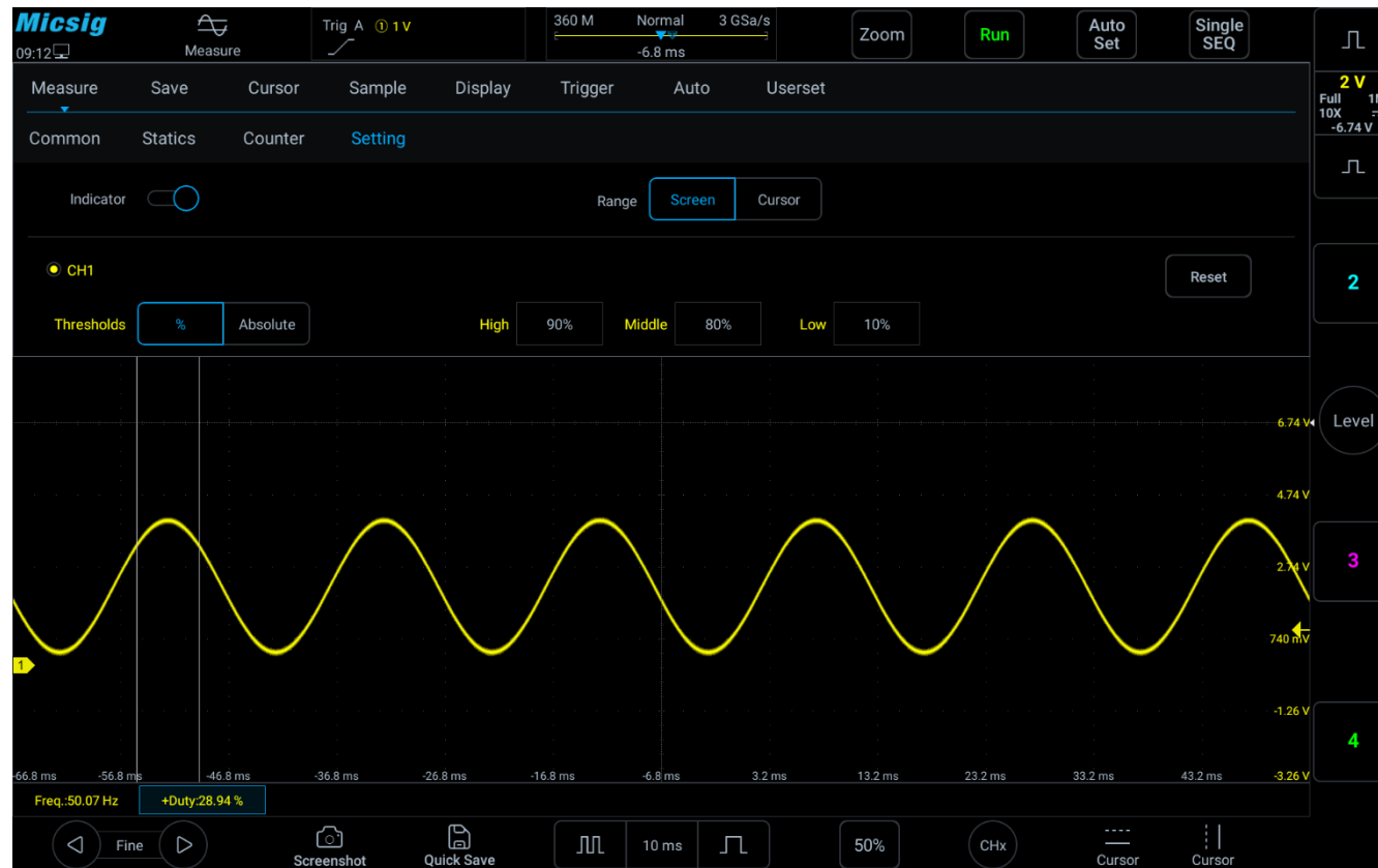
6-13 Pulse width when the median threshold value is set to 80%
