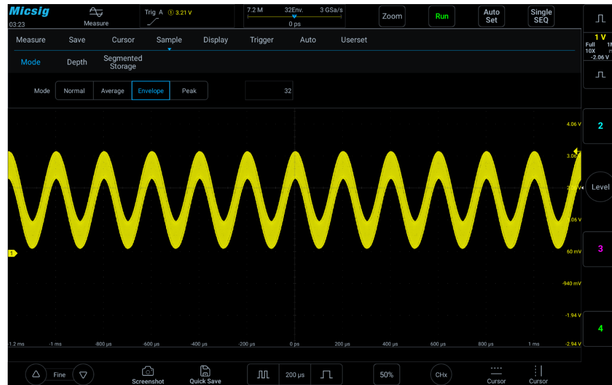
Figure 10-8 Signal in Envelope Sampling Mode (32)
