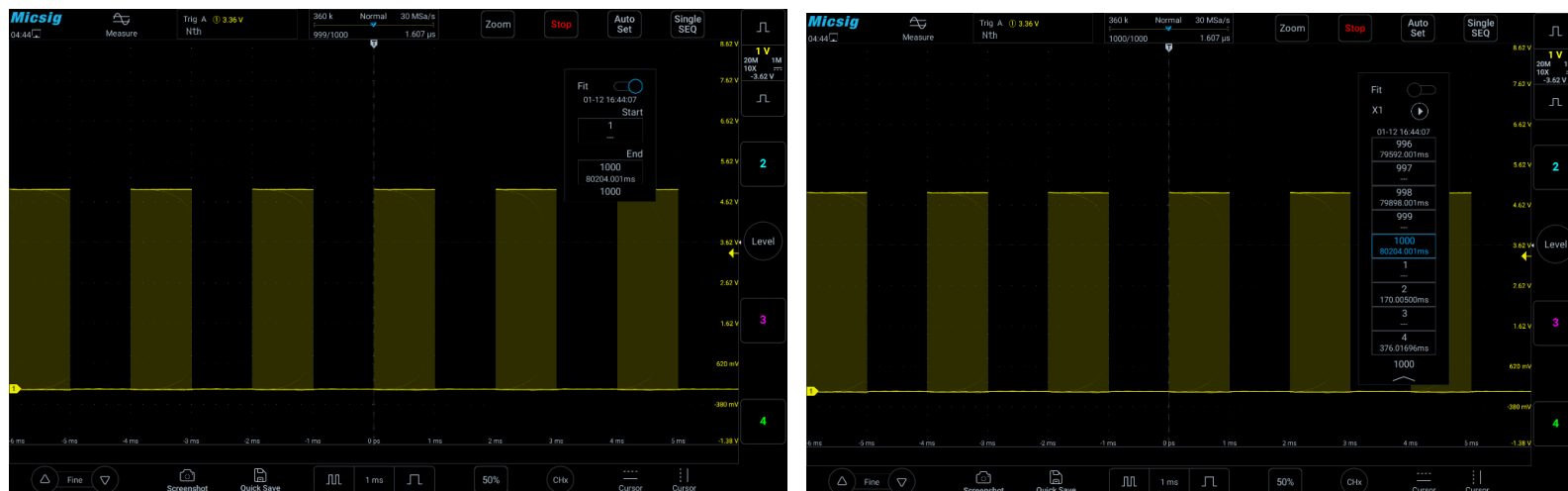
Figure 10-15 View after segment collection is completed
