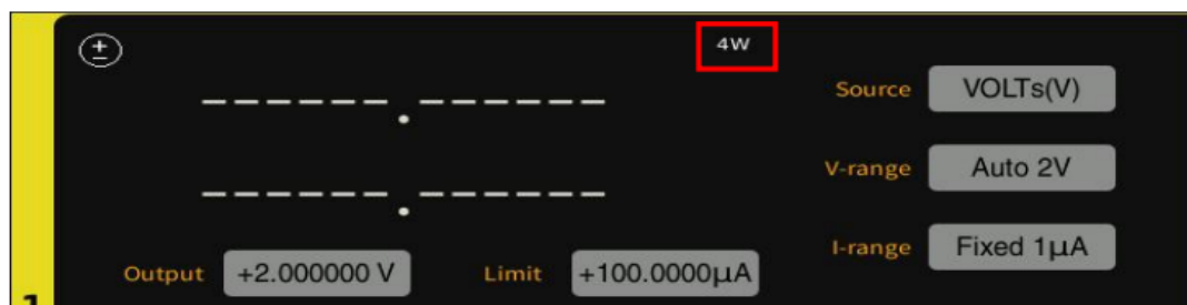
Figure 4-4 Connected 4-Wire Page Display Status
